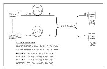
FIGURE 2. Excess & insertion loss measurement - (post-fused)
