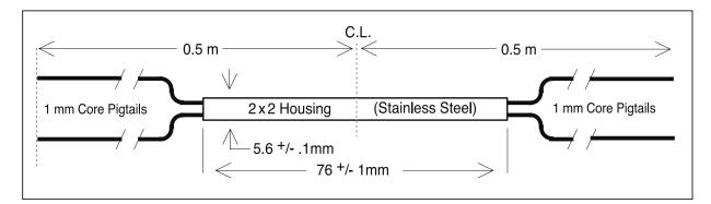
FIGURE 3. Overall Dimensions for  $2 \times 2$  Coupler
