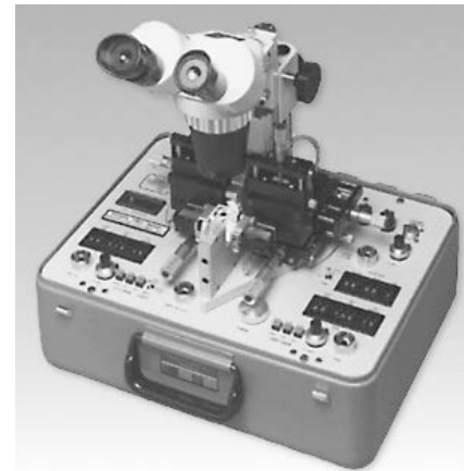
Photo 20. Fusion splice for glass optical fiber.
