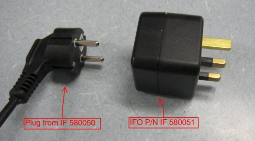
The UK adapter plugs into the wall, the Schuko plug (from transformer) plugs into the adapter.
